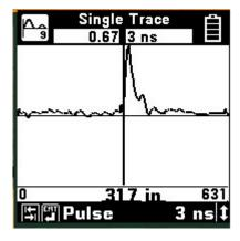
Use the TDR Single Trace mode to test a single coaxial wire or circuit.
